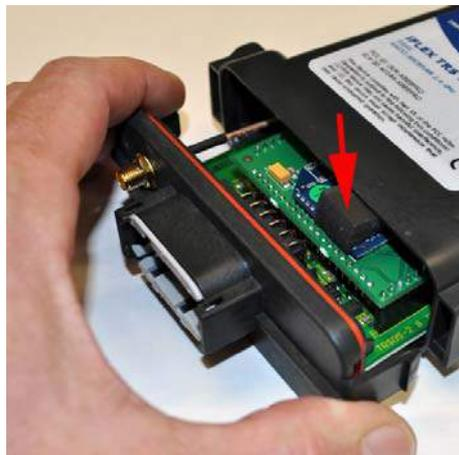
▲ **1.** Carefully slide the circuit board into the guide rails in the housing. Make sure that the foam strip is positioned as shown.
