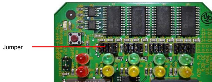
Now set the jumpers **identically for each channel** according to the sketch below:
