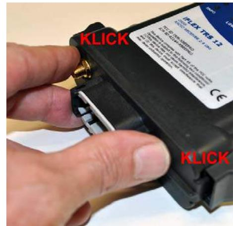
▲ **2.** Lock the circuit board by applying strong pressure to the underside of the housing (clearly audible click at **both** sides).
