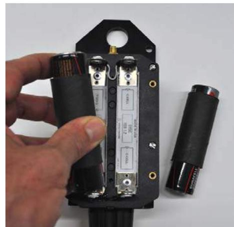
▲ **2.** Remove the batteries
