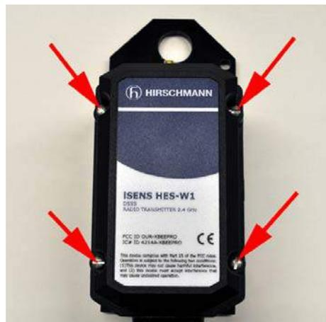
▲ **1.** First of all, open the battery compartment of the **wireless sensor** to be registered by undoing the cover screws and removing the cover of the battery compartment.
