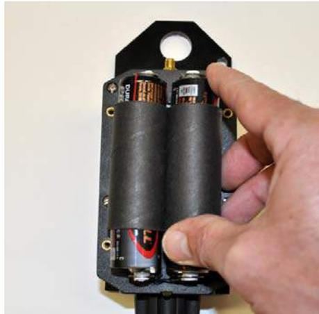
▲ **4.** Now insert the batteries into the battery compartment of the wireless sensor to be registered, observing the correct polarity.
