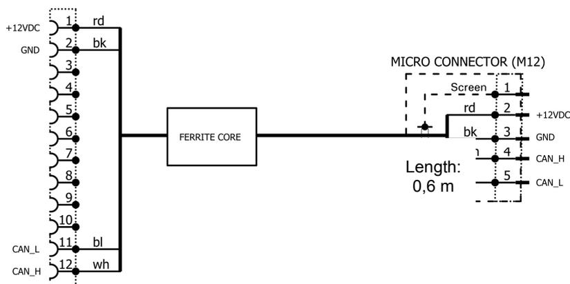
Figure 6: Wiring of the CAN connecting cable
