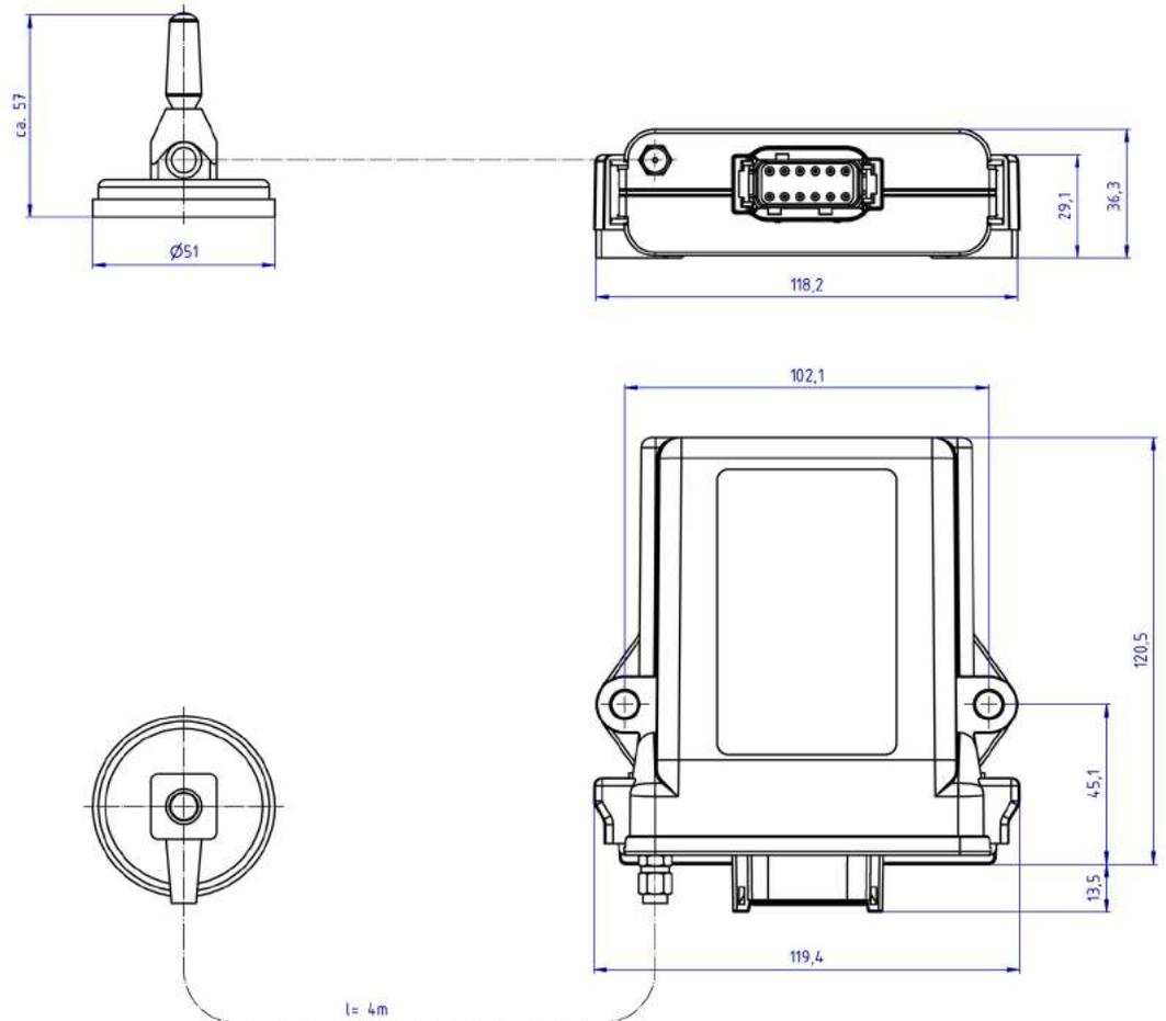
**Figure 2:** Dimensions of the iFLEX TRS 10 (with magnetic base antenna)
