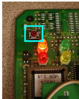
**Figure 10:** Red push button on TRS 10 board
