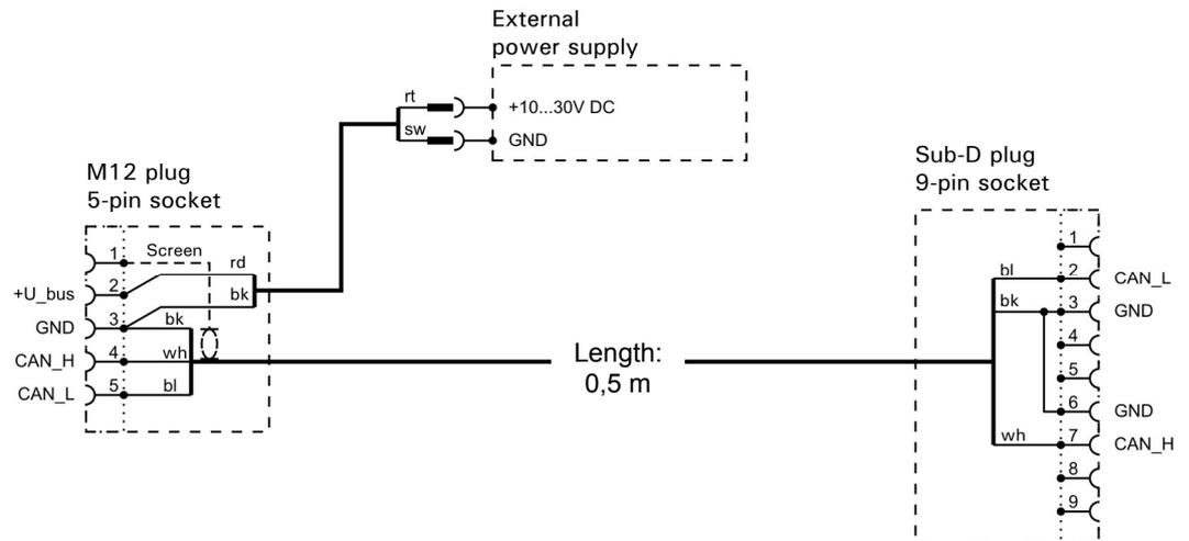
**Figure 11:** Wiring of the adaptor cable for PCAN-USB
