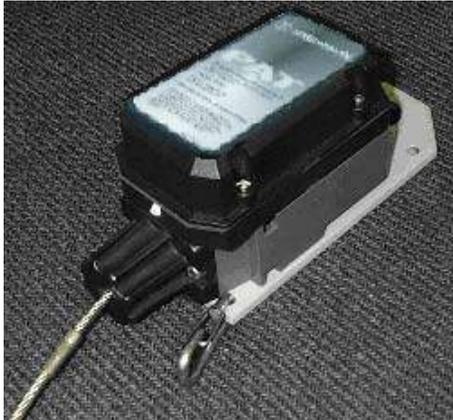
Radio A2B transmitter assembly with antenna
