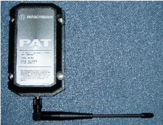
Angle sensor with transmitter
