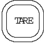
The button "Tare" (9) is used to indicate the net load on the display. Net load is the actual load, less lifting tackle and hook block. The button "Tare" has to be activated before lifting.
